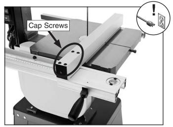
Figure 41. Location of the fence adjustment cap screws.
